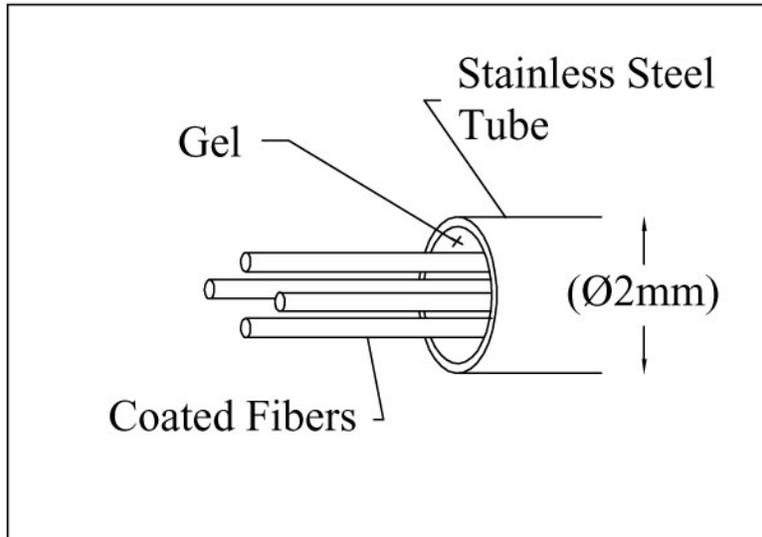
Figure 3 - Multiple optical fibers bundled in a “stainless steel tube”.
