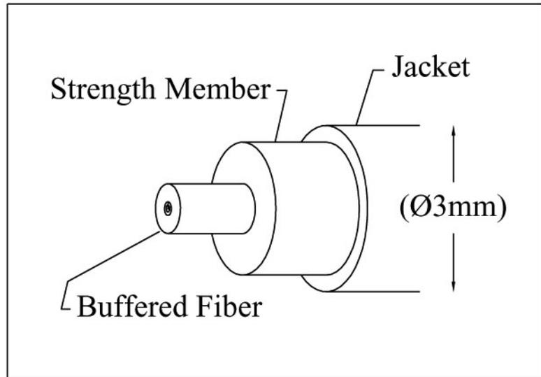
**Figure 2 - The stand-alone optical fiber unit.**
