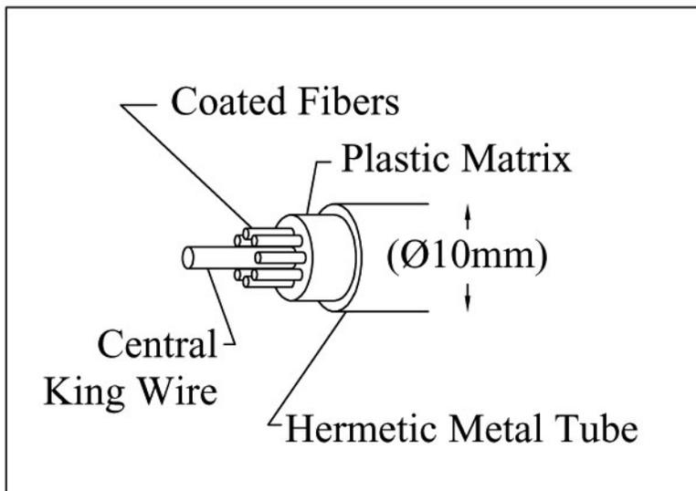
Figure 4 - Multiple optical fibers in an “Embedded Matrix”.
