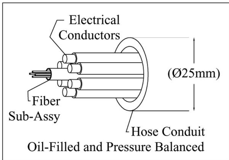
**Figure 6 - Typical oil-filled jumper hose assembly.**
