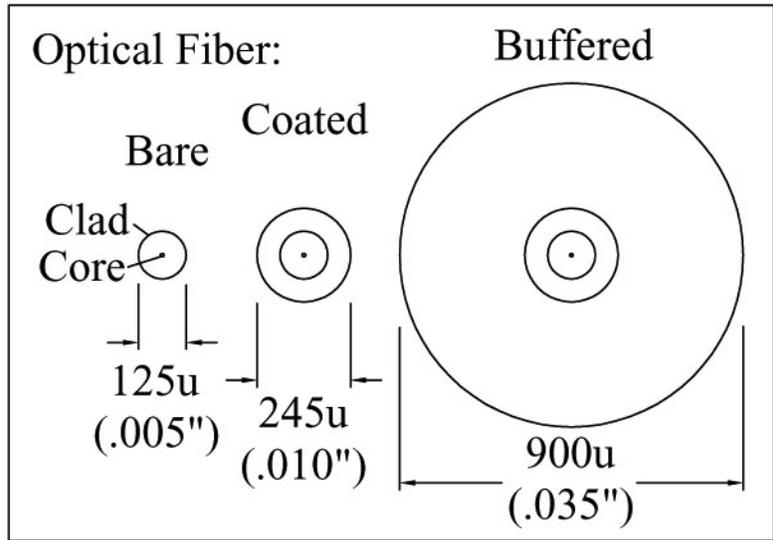
**Figure 1 - Basic optical fiber construction.**
