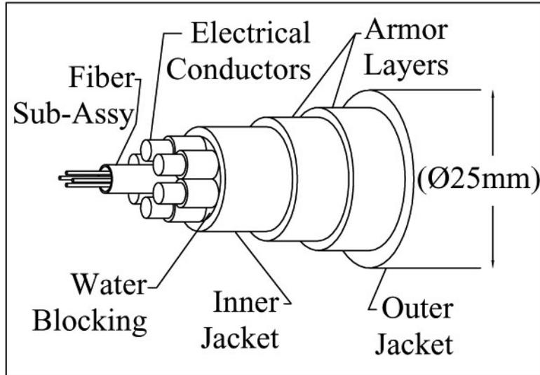
**Figure 5 - Typical oceanographic electro-optical cable.**
