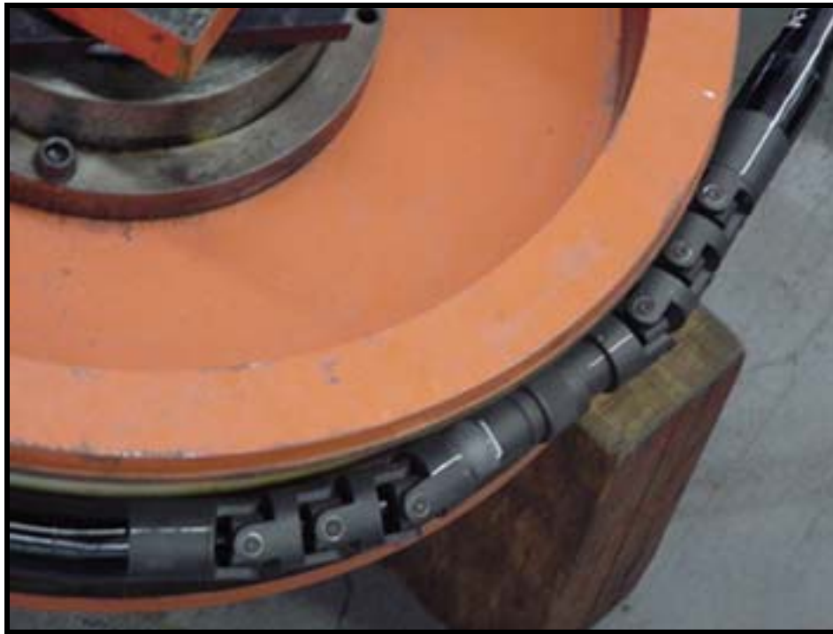
Figure 7 – Dynamic cyclic bend of Universal Joint Bend Restrictor (UJBR) connector over 0.9m (36”) diameter sheave
