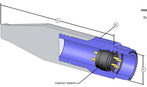
G, K, L, M sizes have round keyway. O, P and Q have square keyway. Refer to pages 11-16 for contact configurations. G, K, L, M Aluminum connectors will not mate with Stainless Steel connectors.
