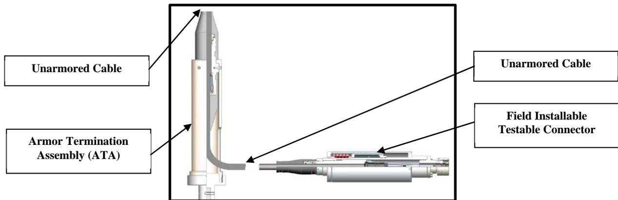
Figure 2 – Separated Cable Termination System
