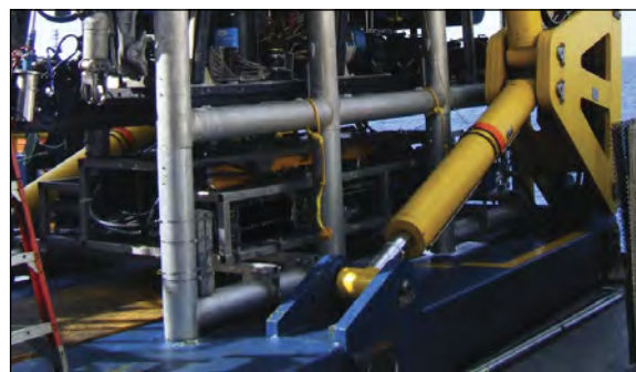
Figure 8: ROV with mounted skid
