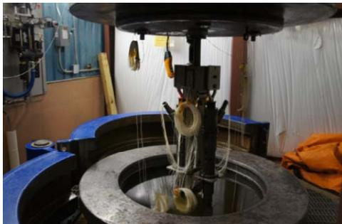
Fig. 6. High Capacity Wet Mateable Optic Connector During Pressure Testing
