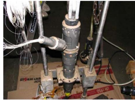
Fig 7. High Capacity Wet Mateable Optic Connector During Following Turbid Tank Testing
