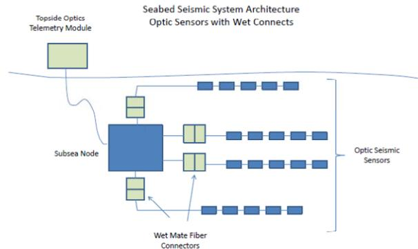
Fig. 8. Seabed Seismic System Architecture Using Optic Sensors and Wet Mate Connectors
