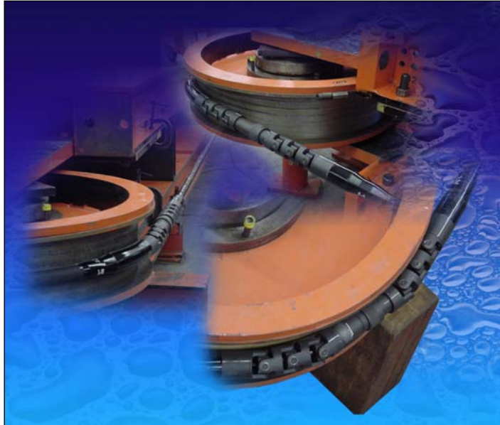
Dynamic cyclic bend of Bend Restrictor connector over 0.9m (36") diameter sheave
